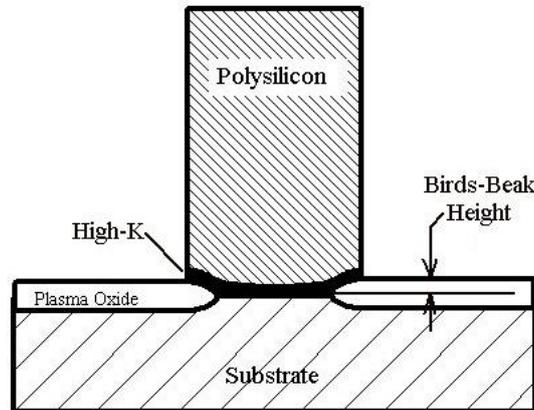
**Fig. 2** Interfacial oxide growth at gate-edge using oxidizing plasmas.
