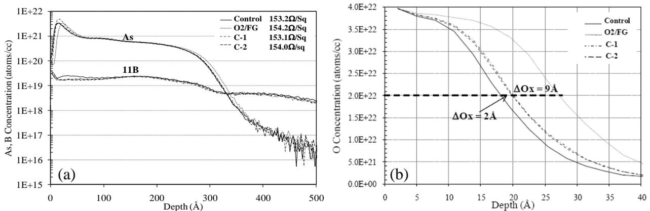
**Fig. 3** SIMS depth profiles: (a) As and B, (b) O.
