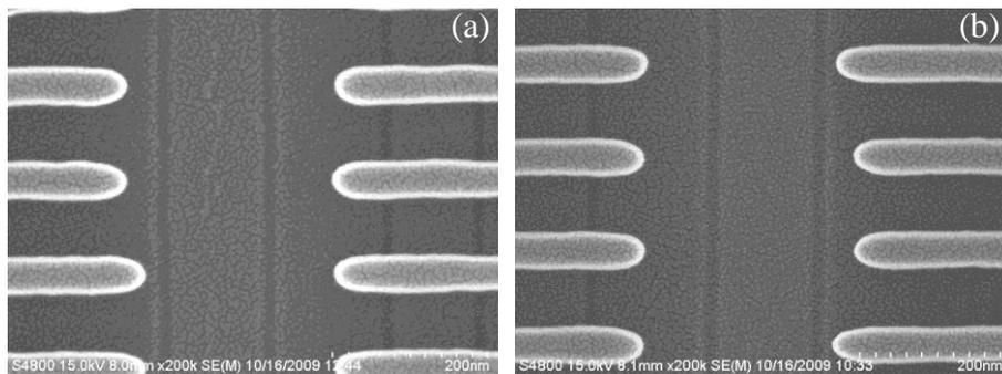
**Fig. 1** Post-strip SEM images of HDIS for post LDD: (a) FG-only, (b) C-2.
