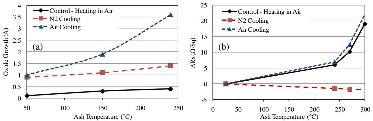
**Fig. 4** Cooling environment effect of post FG-only strip substrate oxidation: (a) Si, (b) TiN.
